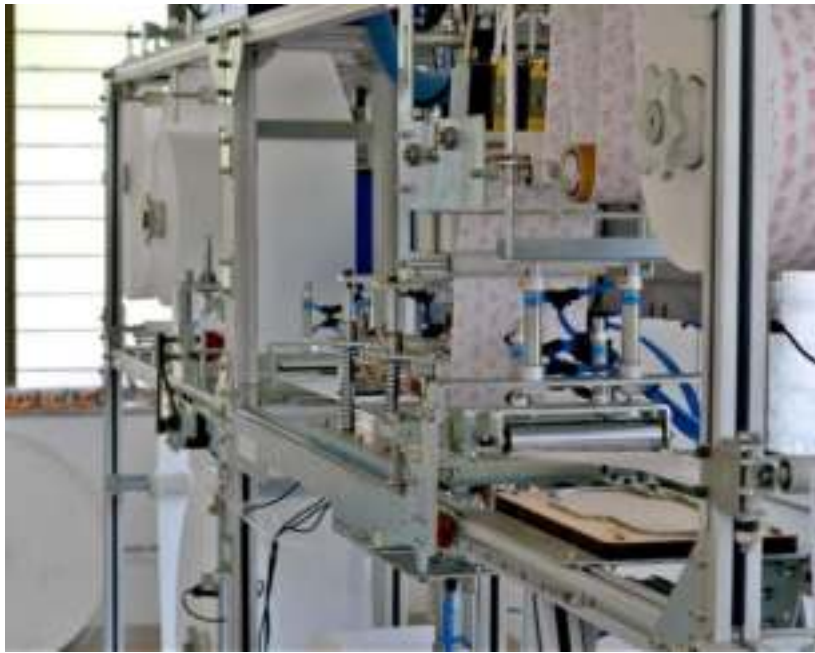
Swachh automatic sanitary napkin-making machine at Saral Design's factory. Photo credit: Sharanya Hariharan.
